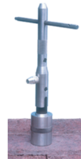
4. Place tool on castle nut and turn clockwise to remove anchor
