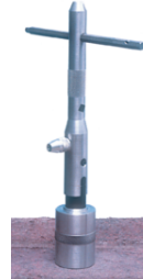
5. Attach tool. Turn clockwise to remove anchor.
